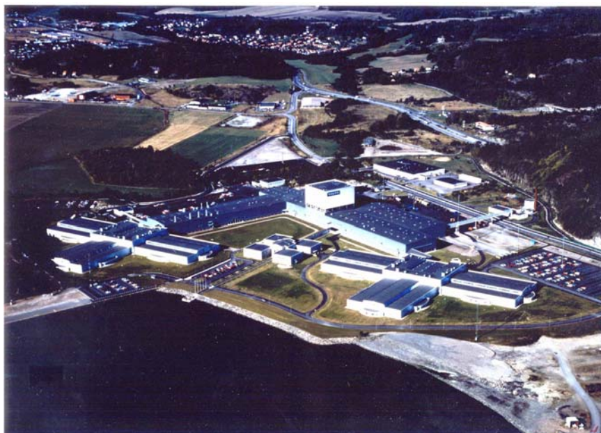
Fig. 3. Aerial view of the Uddevalla plant as build. The two trifoliate buildings, each containing three product workshops, face the sea. Between them, the office building, and behind them, a converted sheet-metal hall used for material stores (1989)
